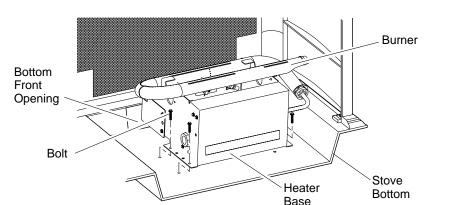
Figure 13 - Placing Heater Base In Stove Cavity (Appearance May Vary Depending on Model)
